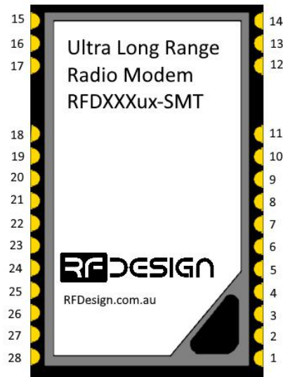
Figure 5- 2: Physical pin layout (top view) of the RFD900ux-SMT/868ux-SMT modem Radio Modem
